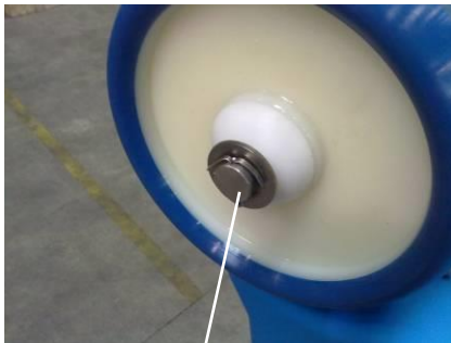
Fixed castor with a plain washer at both sides of the wheel. Split pin for fixation.
