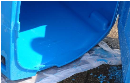
Position of the Drumtainer for optimal drainage
