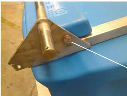
M10 fasteners for the fixation of the frame
