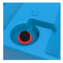
The connector of the low-level sensor (option) has a 2-pin plug. The circuit of the low-level sensor is opened when the level in the VARIBOX CC is low: at approximately 50 litres of remaining content. The sensor opens also when the cable of the switch is damaged. Max. switching voltage is 48 V; max. switching current is 0,5 A. The correct socket for this plug is: Bulgin standard Buccaneer PX0736/S (screw termination, see picture). The sockets are available in the VARIBOX webshop for spareparts.
