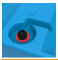
The connector of the empty sensor (option) has a 2-pin plug. The circuit of the empty sensor is opened when the VARIBOX FC is almost empty: at approximately 1 litre of remaining content. The sensor opens also when the cable of the switch is damaged. Max. switching voltage is 48 V; max. switching current is 0,5 A. The correct socket for this plug is: Bulgin standard Buccaneer PX0736/S (screw termination). The sockets are available in the VARIBOX webshop for spareparts.
